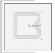
RFID-Codes are located on RFID labels (TAG).
